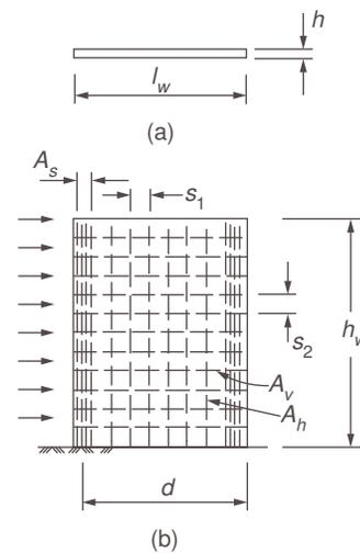
FIGURE 50.31 Geometry and reinforcement of typical shear wall; (a) cross section; (b) elevation.
