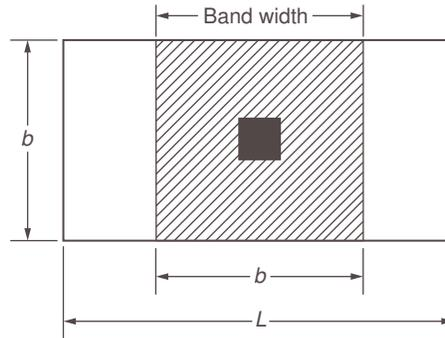
FIGURE 50.21 Band width for reinforcement distribution. (Source: MacGregor, 1992.)
