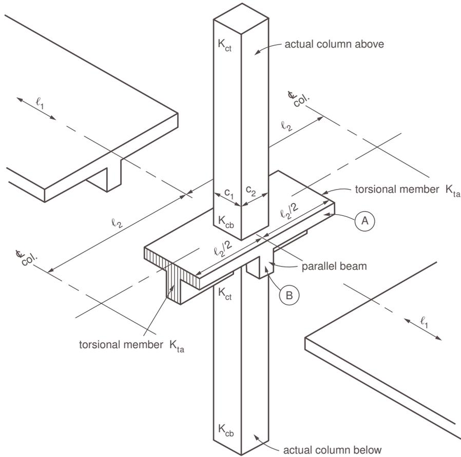
FIGURE 50.7 Equivalent column (columns plus torsional members).
