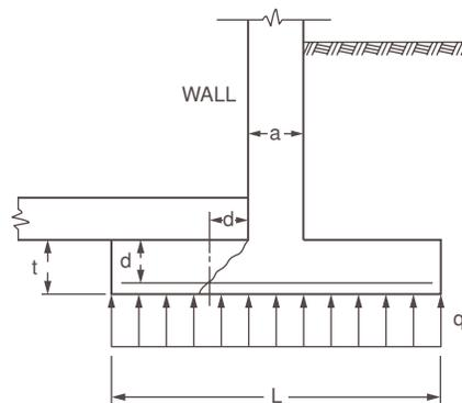
FIGURE 50.23 Reinforced-concrete wall footing. (Source: Wang and Salmon, 1985.)
