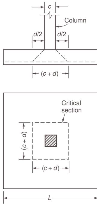
**FIGURE 50.18** Punching shear (two-way).
