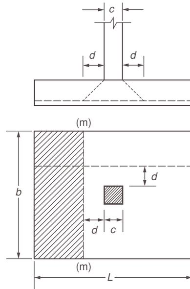
**FIGURE 50.19** One-way shear. (Source: MacGregor, 1992.)
