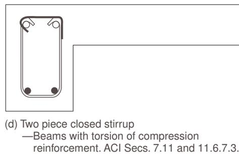
FIGURE 50.4 Stirrup detailing requirements. (Source: Wang and Salmon, 1985.)
